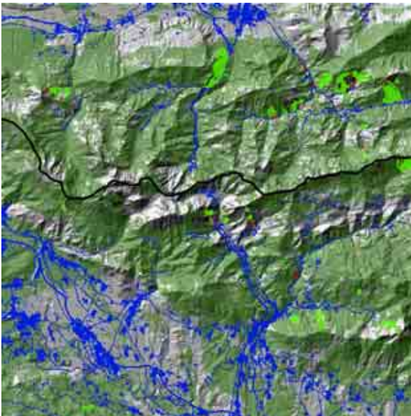
Figure 5-63: Cross border test site C4-1 Austria – Slovenia. Dark green – Forest map; light green – RPF; red – RPF with width < 200m; blue – Infrastructure in parts of the test site C4 – Slovenia.
