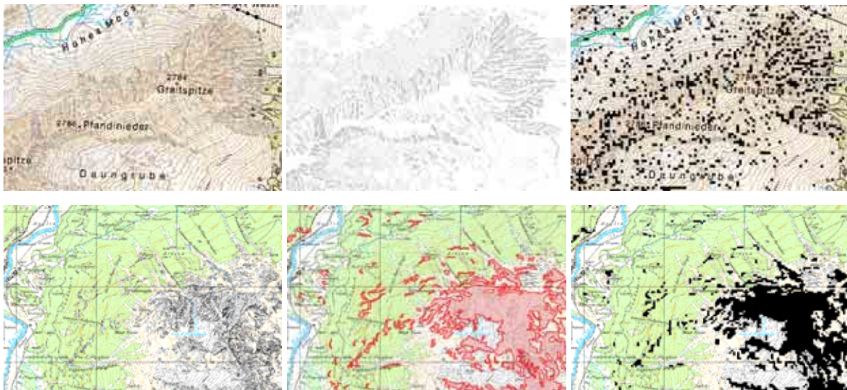
Figure 5-35: Top: Austria - Example of OEK50 – extracted rock layer – final rock mask. Bottom: Switzerland - Example of Vektor25 – selected rock polygon – final rock mask.
