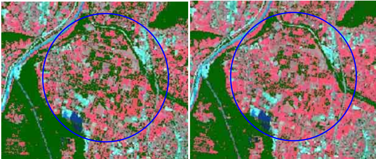
Figure 5-17: Example of misclassified area: results using Swiss data only (left) and Austrian data only (right); parts of fields are always classified as forest
